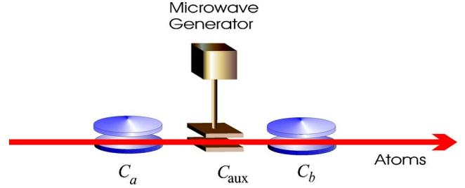
FIG. 2. (Color online) Experimental setup for probing finite-time decoherence in cavity QED.
