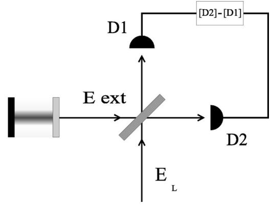
FIG. 1. Homodyne scheme. The intracavity field leaks through the semitransparent mirror and is mixed with the local oscillator field at the beam splitter. The signals detected at  $D1$  and  $D2$  are subtracted.
