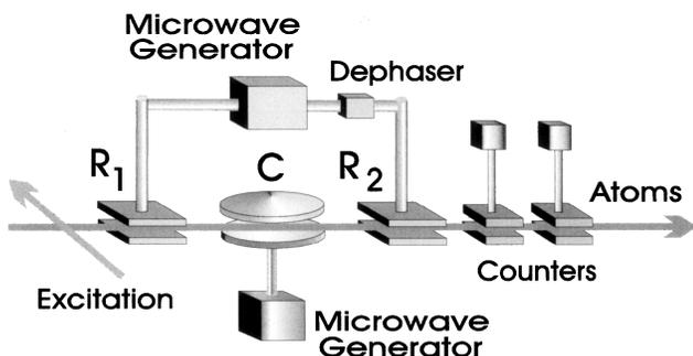
FIG. 1. Cavity QED experiment for measuring the Wigner function of an electromagnetic field in cavity  $C$ .
