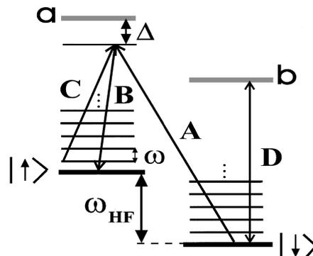
FIG. 3. Trapped ion: relevant level scheme (not in scale).
