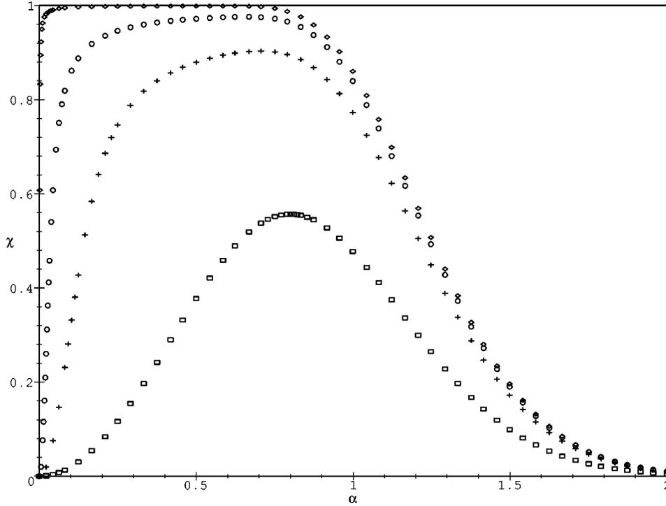
FIG. 4. Squeezing as a function of  $\alpha$  when the number of detected atoms is  $N=1$  (squares);  $N=3$  (crosses);  $N=5$  (circles), and  $N=10$  (lozenges). As the number of detected atoms increases, the squeezing becomes quite insensitive to the value of  $\alpha$ .
