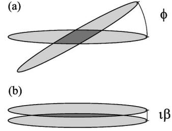
FIG. 8. The probability difference  $\Delta P$  is sensitive to the overlap between the field distributions before and after interacting dispersively with a probe atom. (a) Rotational width can be measured by a rotation by  $\phi$ . (b) Translational width is measured by a state-dependent displacement  $i\beta$  of the field.
