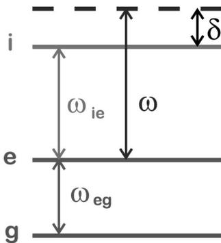
FIG. 2. Atomic level scheme. The transition  $i \leftrightarrow e$  is detuned by  $\delta$  from the frequency  $\omega$  of a mode of cavity C, while the transition  $e \leftrightarrow g$  is resonant with the fields in  $R_1$  and  $R_2$ . State  $|g\rangle$  is not affected by the field in C.
