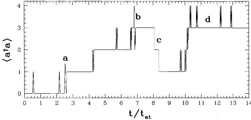
FIG. 1. Single realization of a Poissonian-pumped micromaser with collective effects. The initial state of the field is the vacuum, which is a trapping state. The temperature and the velocity dispersion are zero, the field profile is constant, and the incoming atoms are excited and resonant with the cavity mode. The dashed lines correspond to quantum jumps. Here  $N_{\text{ex}}=10$  and the average number of atoms in the cavity is  $N=0.1$ .
