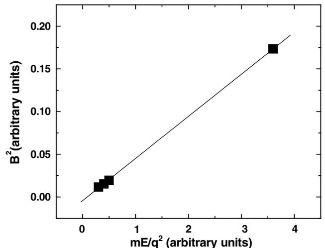
Fig. 2. Calibration of the switching magnet.
