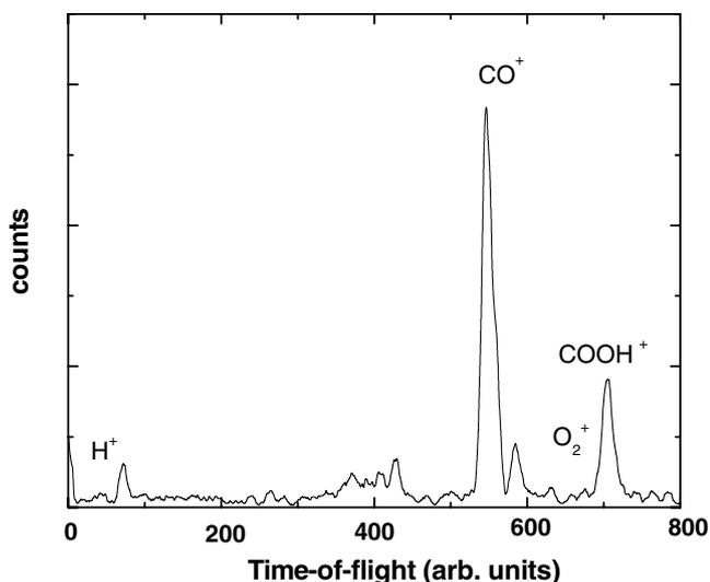
Fig. 5. A time-of-flight mass spectra of formic acid ionized a by 2.0 MeV  $p^+$  impact.
