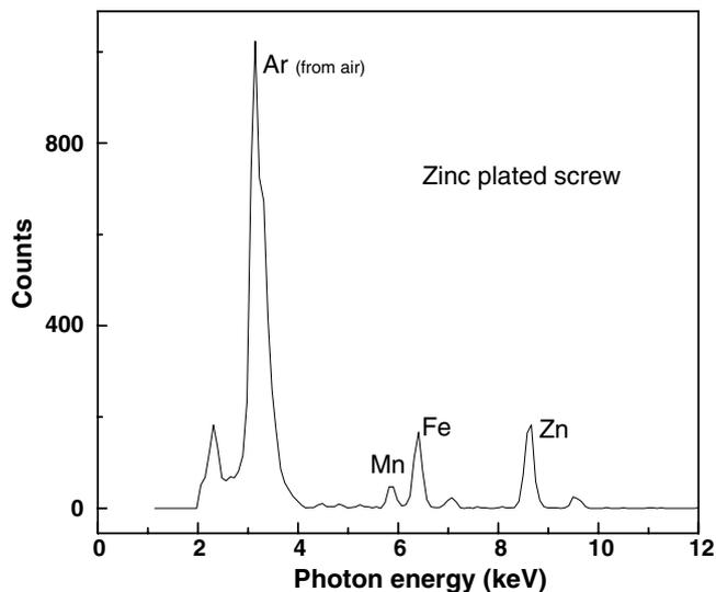
Fig. 6. PIXE spectrum of a zinc plated screw.
