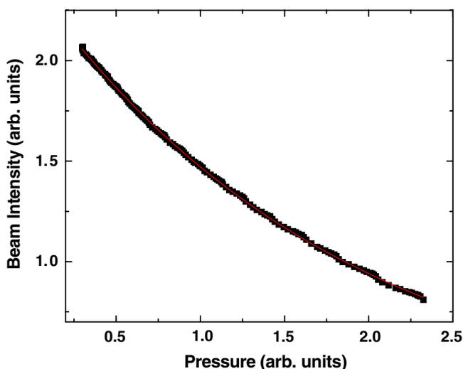
Fig. 4. Typical beam attenuation curve for a 400 keV Cl beam. The solid line is the exponential fit to the data, from which the value of the detachment cross-section is obtained.
