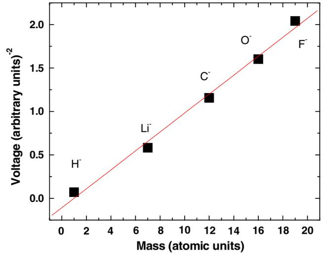
Fig. 1. Mass spectrometry of negative ions from the SNICS source using a Wiens filter.
