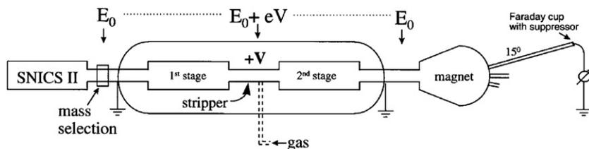
Fig. 3. Schematic diagram of the accelerator.
