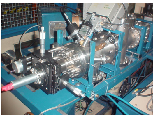
Figure 2. Detail showing the home-made MALDI camera and the laser.
