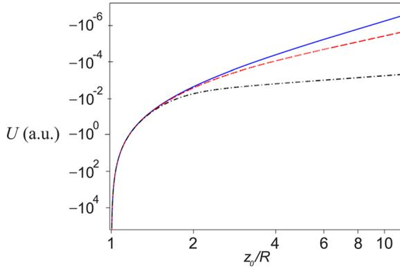
Fig. 4. (Color online) Exact expressions for  $U_{ags}$  (blue solid line) and  $U_{abh}$  (dashed red line), given by Eqs. (30) and (49), respectively, and an expansion up to second order for  $U_{ags}$  (dotted-dashed black line), obtained from Eq. (54), as functions of  $z_0/R$ . Both axes use logarithmic scales and arbitrary units.
