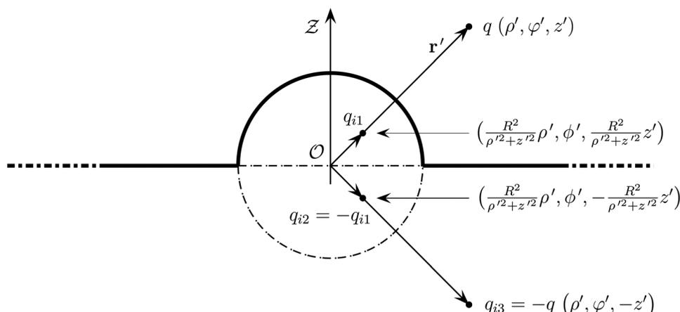
Fig. 2. Charge  $q$  near a conducting boss hat surface and its three image charges.
