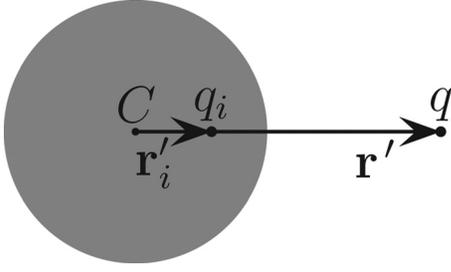
Fig. 1. Point charge  $q$  near a grounded conducting sphere of radius  $R$  and its image  $q_i$ .
