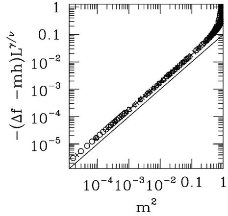
FIG. 6. Negative Gibbs free energy  $-g = -(\Delta f - mh)$  times  $L^{\gamma/\nu}$  against  $m^2$  for pure Ising systems at criticality. For a key to the symbols, see the caption of Fig. 5. The straight line has a unitary slope, and is a guide to the eye. Normalized magnetizations on the horizontal axis only.
