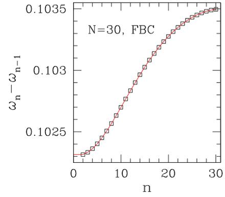
FIG. 2. (Color online) Ising strips with FBC and isotropic interactions, at  $T_c$ : differences  $\omega_n - \omega_{n-1}$  ( $n \geq 2$ ) between consecutive solutions of Eqs. (26) and (27), for strip of width  $N = 30$  sites.
